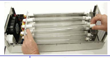
5a. To remove the lower level of tubes on the UV 2700 simply remove the ties and tubes as in step 4.
